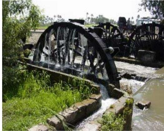
*Self operating device pumping water continuously using the running water to rotate the wheel*
